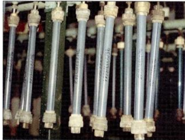
Pipes during main test in pressure resistance test At 20°C in water/in air
